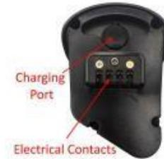
Fig. 17 Charging Port and Electrical Contacts
